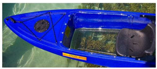
The Caribe is half sit-on-top kayak, half canoe The crystal clear hull of the Caribe provides a window to the underwater world. Based on hull shape it has a remarkable tracking ability and it is very stable.
